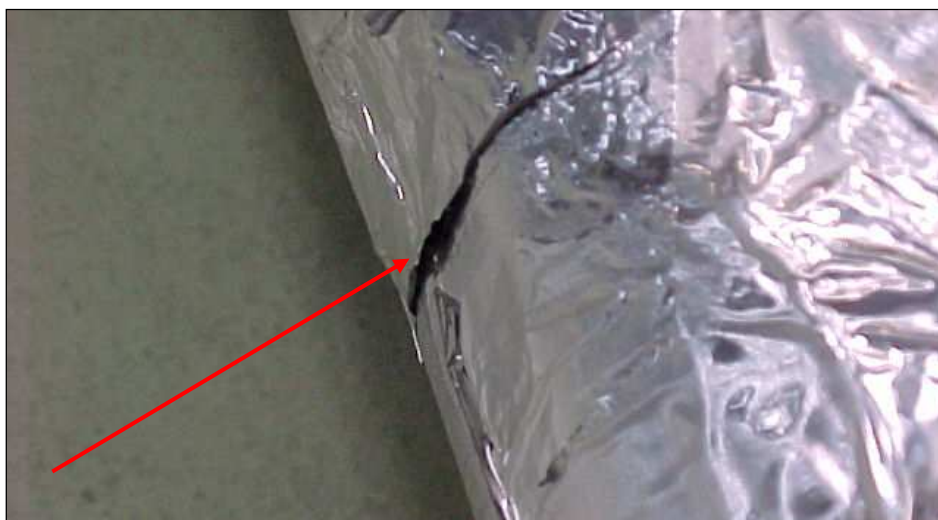
Adhesive tape begins to peel off – P5858 sample
