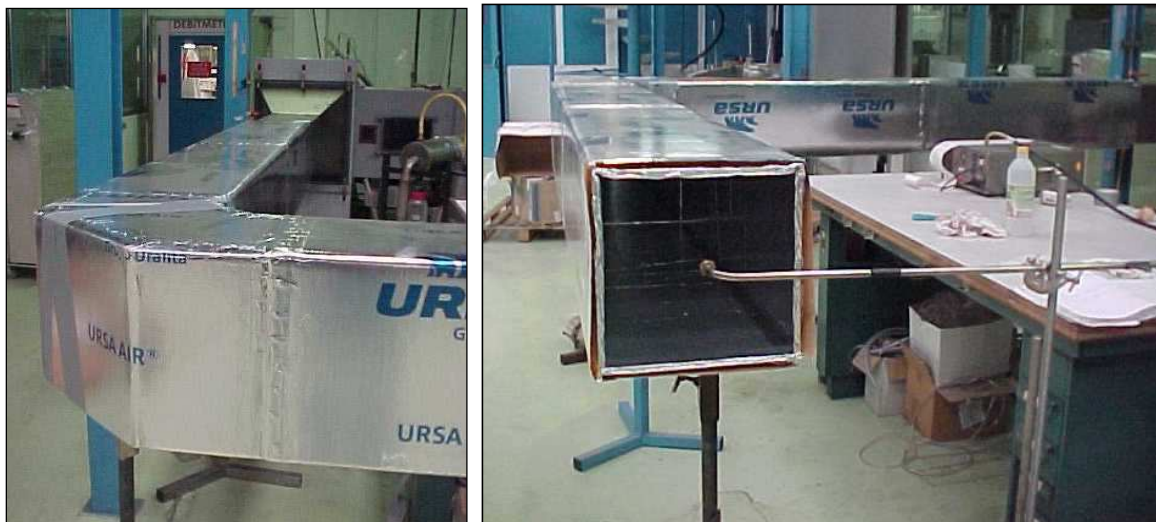
Views of the installation with the tested ducts
